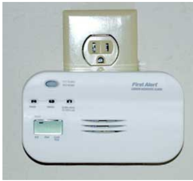
Simple Carbon Monoxide alarms can be purchased and easily installed in an outlet near the heater.
